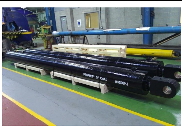
Hydraulic cylinders for linkspan
