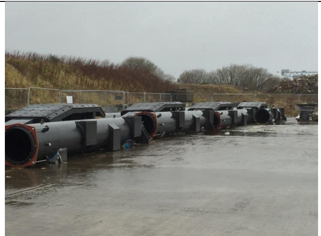
Fender assembly completed at Inchgreen
