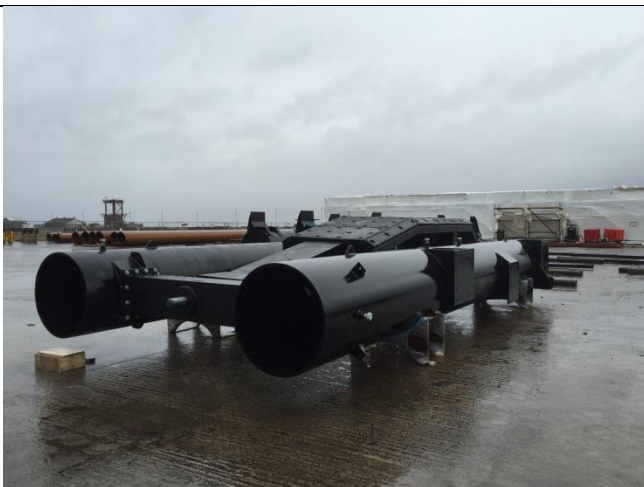
Close up of fender sleeves and pivot fender
