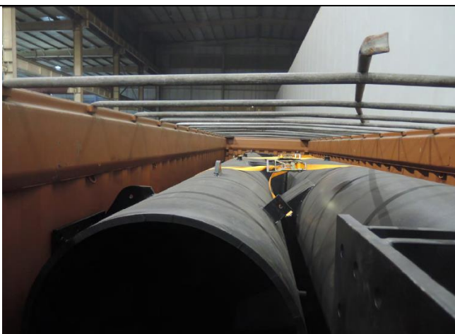
First fender shipment being packed at factory ready for shipment- fender pile steel sleeves
